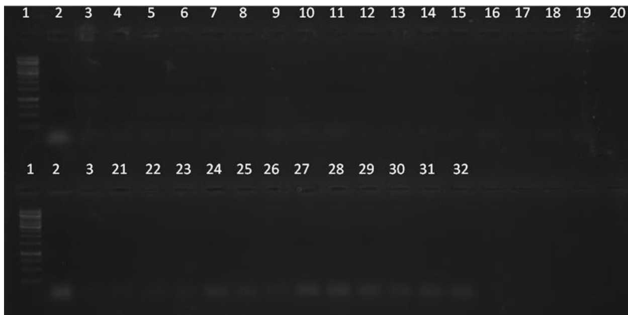
Fig 1. DNA interaction studies using gel electrophoresis of ligands and their metal complexes (at 10 \mu M conc.); 1 = ladder, 2 = DNA ( Micrococcus luteus ), 3 = blank, 4 = \text{CrCl}_3 , 5 = \text{Cr}(\text{OAc})_3 , 6 = \text{Co}(\text{OAc})_2 , 7 = \text{Ni}(\text{OAc})_2 , 8 = \text{CuCl}_2 , 9 = \text{Cu}(\text{OAc})_2 , 10 = \text{ZnCl}_2 , 11 = L1, 12 = \text{Cr}[\text{L1}]_2 , 13 = \text{Cr}[\text{L1}]_2 \cdot 2\text{H}_2\text{O} , 14 = \text{Co}[\text{L1}]_2 , 15 = \text{Ni}[\text{L1}]_2 , 16 = \text{Cu}[\text{L1}]_2 , 17 = \text{Zn}[\text{L1}]_2 , 18 = L2, 19 = \text{Cu}[\text{L2}]_2 , 20 = \text{Zn}[\text{L2}]_2 , 21 = L3, 22 = \text{Co}[\text{L3}]_2 , 23 = \text{Zn}[\text{L3}]_2 , 24 = L4, 25 = \text{Cu}[\text{L4}]_2 , 26 = \text{Zn}[\text{L4}]_2 , 27 = L5, 28 = \text{Cu}[\text{L5}]_2 , 29 = \text{Zn}[\text{L5}]_2 , 30 = L6, 31 = \text{Cu}[\text{L6}]_2 , 32 = \text{Zn}[\text{L6}]_2 .
