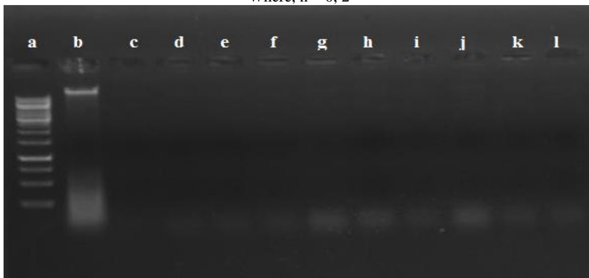
Fig 1. DNA interaction studies using gel electrophoresis of ligands and their metal complexes (at 100 \mu M conc.); a = Ladder, b = prokaryotic DNA, c = Cr(OAc) 3 , d = ZnCl 2 , e = Ni(OAc) 2 , f = CoCl 2 , g = CrL 2 , h = CuL 2 , i = ZnL 2 , j = NiL 2 , k = L1, l = L2
