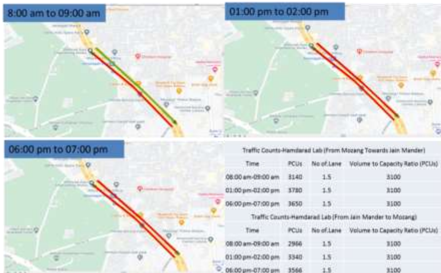
Fig.9. Spatio-Temporal Traffic congestion Status at Lytton Road Corridor
