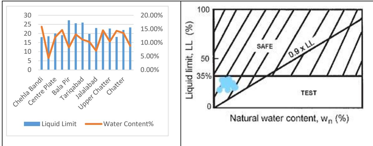
Fig. 2 Liquefaction Susceptibility Criteria proposed By Wang (1979)
