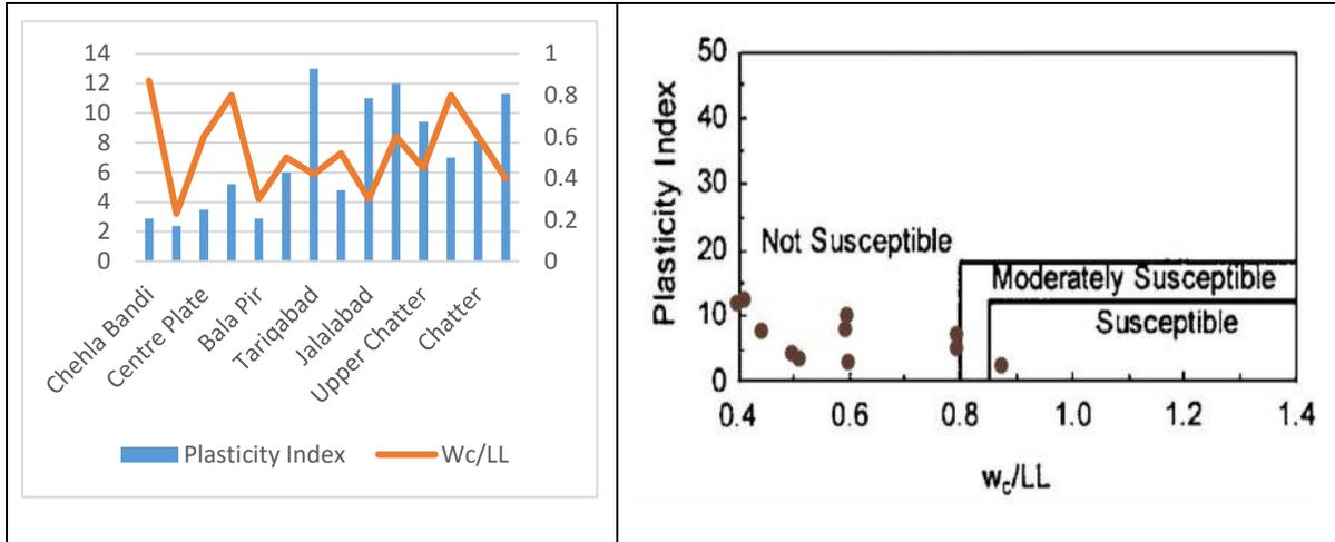
Fig. 4 Liquefaction susceptibility Criteria proposed by Bray & Sancio (2006)
