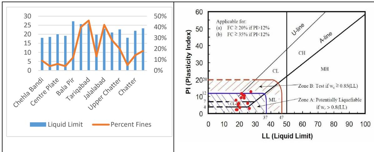
Fig. 3 Liquefaction Susceptibility Criteria Proposed by Seed & Idriss (1982)
