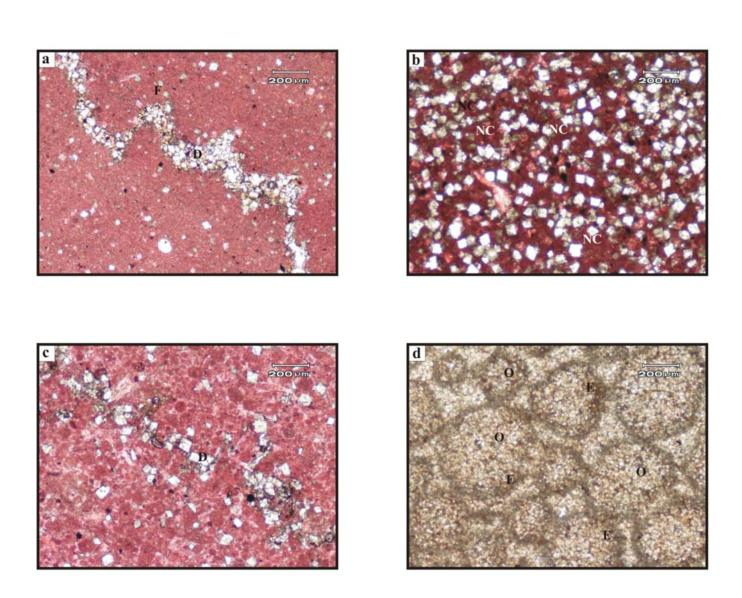
**a.** Photomicrograph showing stylolite along with dolomite stylocummulate **(D)** in a partially dolomitized mudstone. (PPL, stained) **Sample No. SBH-13B**
