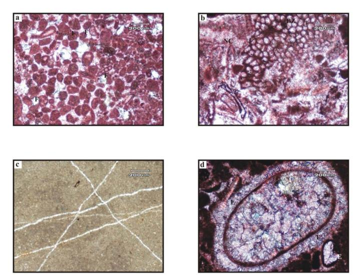
a. Photomicrograph displaying a peloidal grainstone with associated foraminiferal (F) tests. The intergranular drusy mosaic (DM) cement has partially altered into ferroan calcite with light royal blue stain colour. (PPL, stained) Sample No. SBH-74B
