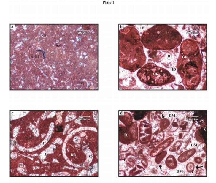
a. Photomicrograph showing peloidal packstone, wherein skeletal grains of echinoderm (EC) and mollusks (M) in association with peloids are present. (XN, stained) Sample No. SBH-23B
