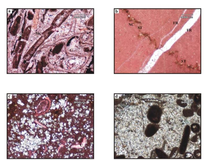
a. Photomicrograph showing a bioclastic rudstone, wherein mechanical compaction (MC) prior to cementation is exhibited by broken algal (A) shells. A large gastropod (G) shell is present too. (PPL, stained) Sample No. SBH-31
