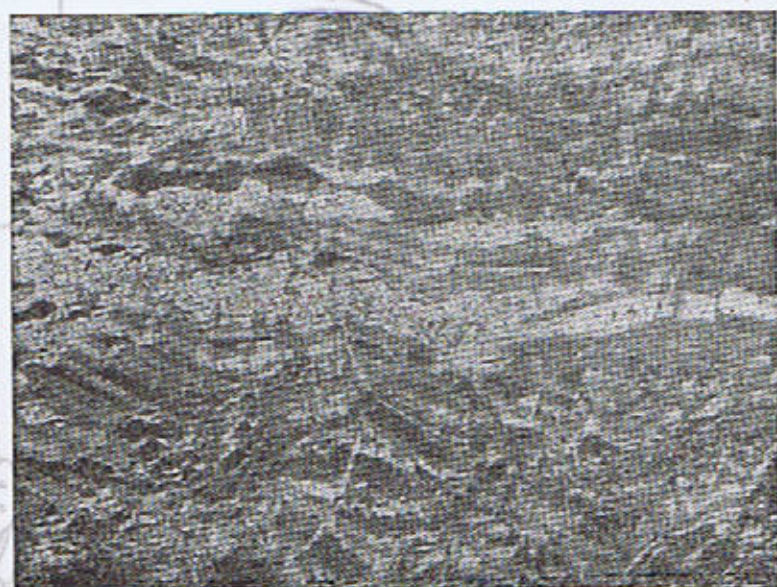
Fig. 6 Sheared (a) tear-faulted and bondinaged (b) aplites in the contact zone near Gamian Sari (dj : diagonal joint).
