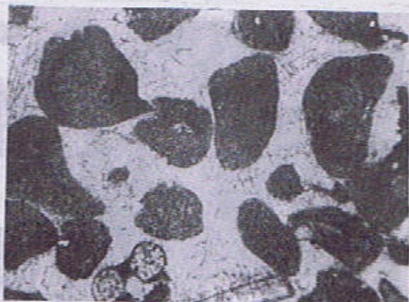
Fig.13 Coarse lithoclastic rudstone-oolitic pelsparite (PPL; 4x; F.V. 1.74 mm).
