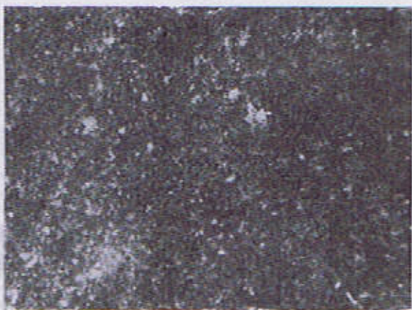
Fig.12 Homogenous unfossiliferous mudstone (PPL; 4x; FV. 1.74 mm).
