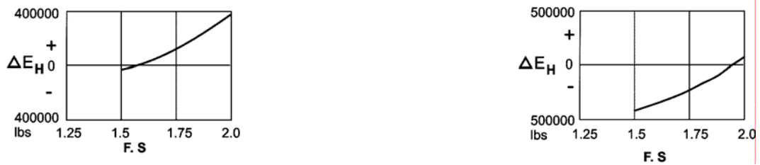
Fig. 4c: Trial Factor of Safety (F.S.) versus Net Effective Force ( \Delta E_H ) to obtain the value at which \Delta E_H=0
