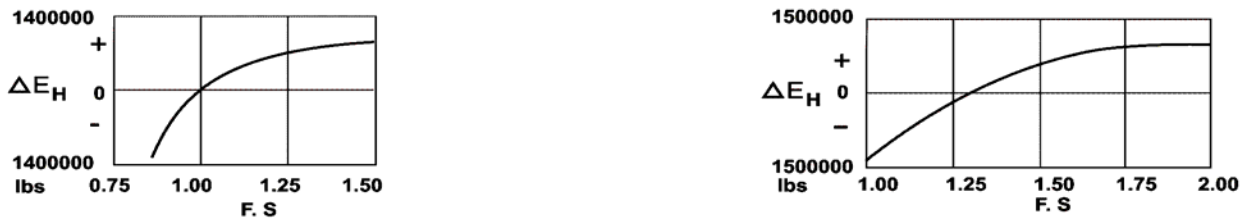
Fig. 6c: Trial Factor of Safety (F.S.) versus Net Effective Force ( \Delta E_H ) to obtain the value at which \Delta E_H=0
