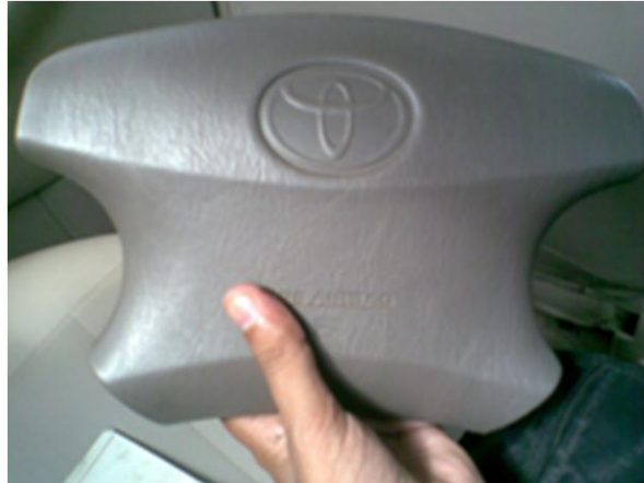
Figure 3: Air bag cover disassembled from steering
