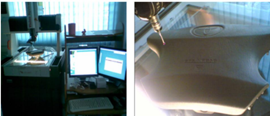
Figure 5: Measuring the four plan sides of air bag cover on CMM
