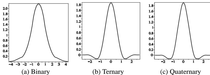
FIGURE 1. (a)-(c) show the basic limit functions of proposed 4-point binary, ternary and quaternary subdivision schemes.
