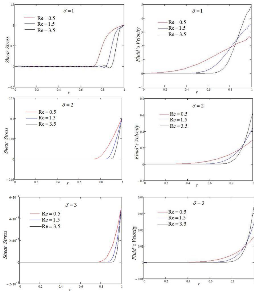
FIGURE 2. Profiles of shear stress and velocity versus  $r$  for  $Re$  variation and different values of  $\delta$ .
