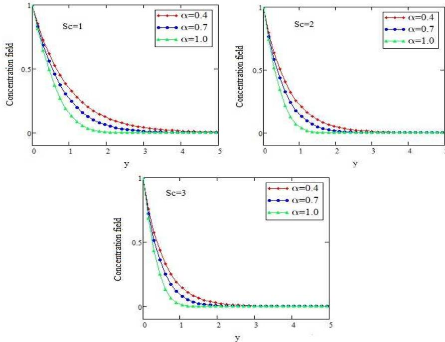
Figure 13: Profiles of concentration field with various values of fractional parameter and Schmidt number  $Sc = 1, 2, 3$ .
