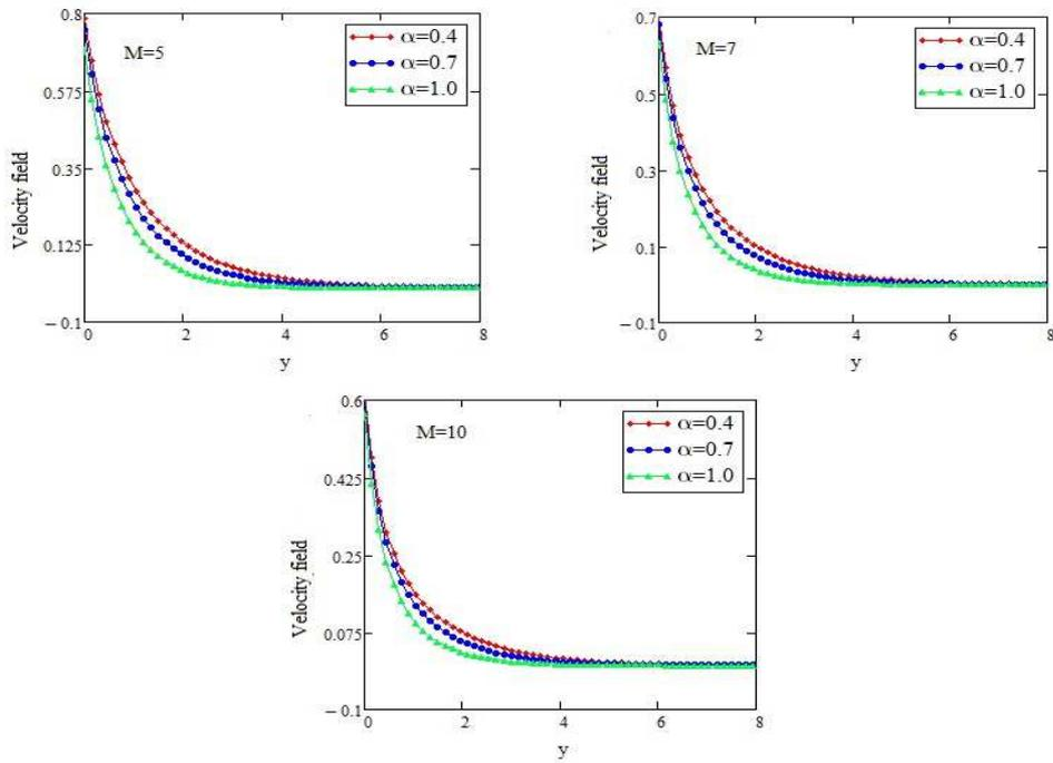
Figure 10: Velocity field representation with various values of  $\alpha$  and magnetic parameter  $M = 5, 7, 10$ .
