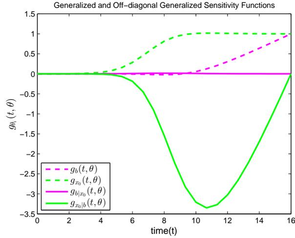
FIGURE 4. Generalized and the off-diagonal generalized sensitivity functions for the selected parameters of the logistic growth population model.
