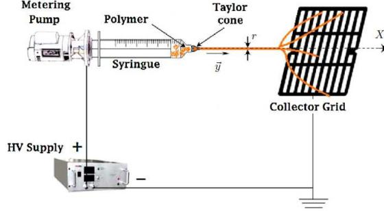
FIGURE 1. Electro-spinning process setup.
