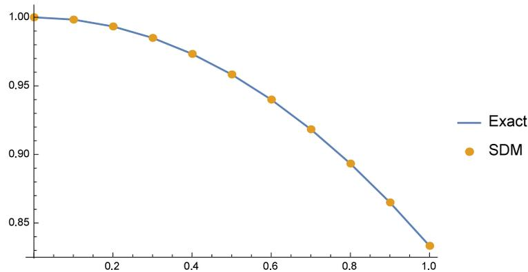
FIGURE 1. Graphical comparison between exact polytropic solution and series solution of case I at  $n = 0$ .
