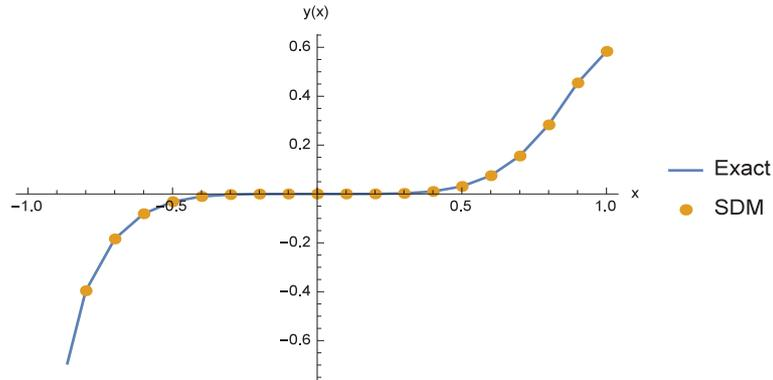
FIGURE 1. Numerical solution obtained from SDM of example 3.1.1 and its comparison with exact solution to verify the accuracy of SDM.
