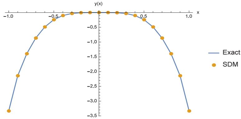
FIGURE 9. Numerical solution obtained from SDM of example 3.3.1 compared by its exact solution to verify the accuracy of SDM.
