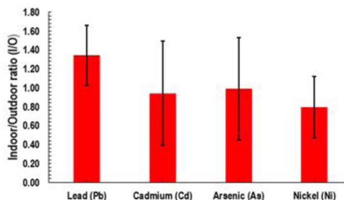
**Figure 2: Indoor/Outdoor ratio of airborne metals in the indoor and outdoor environment.**
