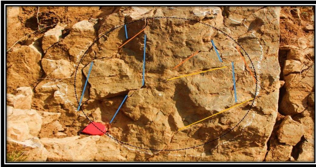
**Fig. 6** Fracture pattern and their sets within circle-2 drawn on Lockhart limestone.
