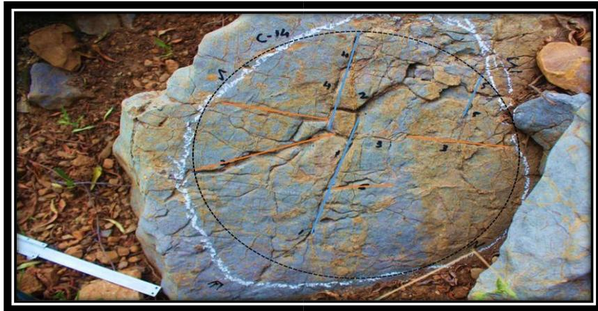
Fig. 12 Fracture pattern and their sets in circle-5.
