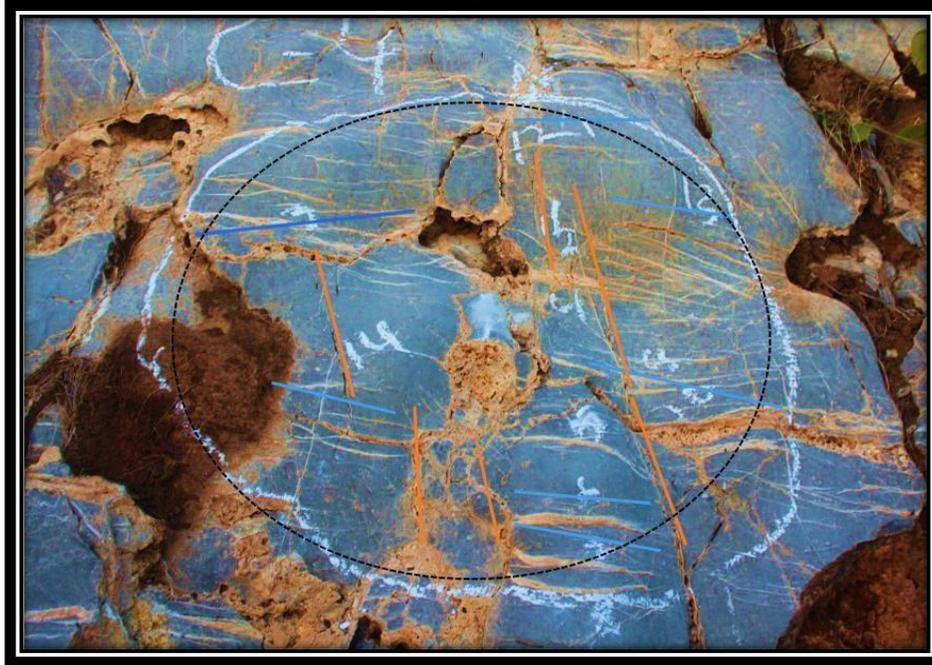
Fig. 4 Fracture pattern and their sets within circle 1.
