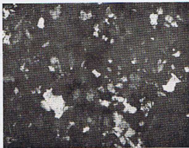
Fig. 5 Photomicrograph of Fine-Grained Albitite Occurring in the Metamorphics at a Distance of about 800 Metres from the Contact of Granite and Metamorphic Rocks. (X 60, x.p.)
