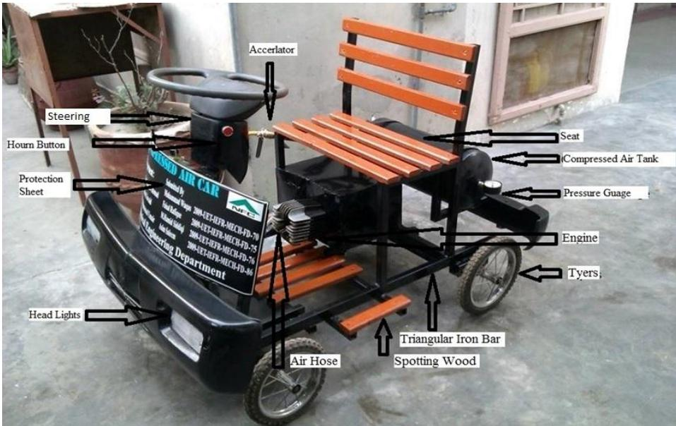
Figure 6: Basic components of Car
