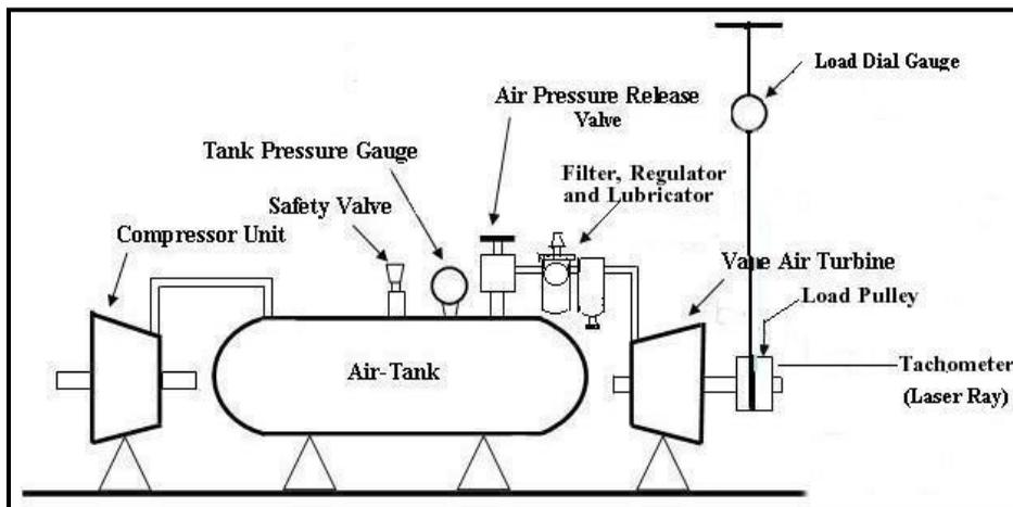
Figure 3: Experimental Test Setup
