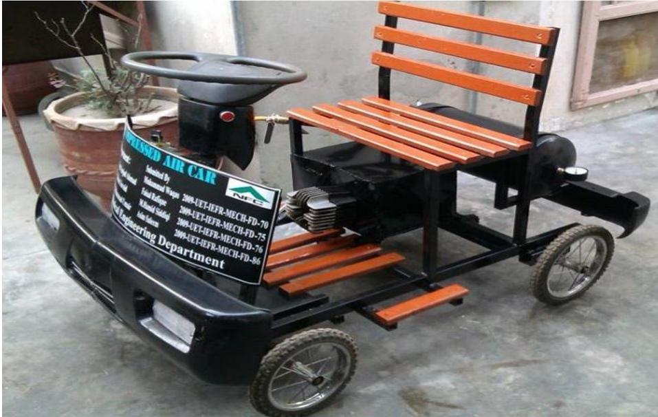
*Figure 4: Assembled Compressed Air Car*
