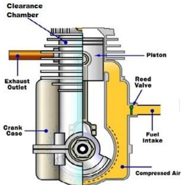
Figure 7: Basic Components of two-stroke Engine
