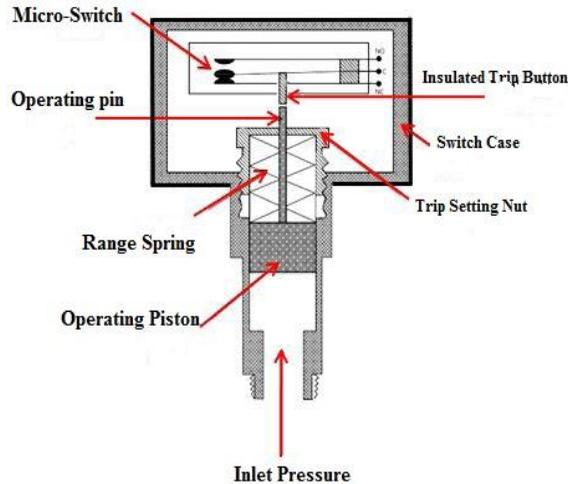
*Figure 9 Sectional view of Pressure Switch.*
