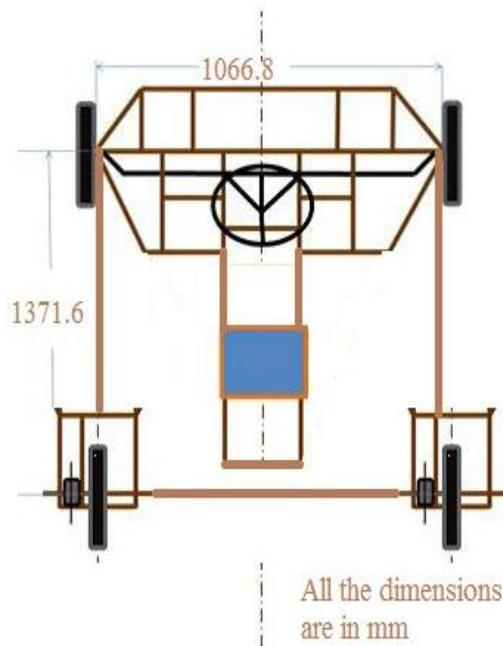
Figure 8: Frame Model of Compressed Air Car
