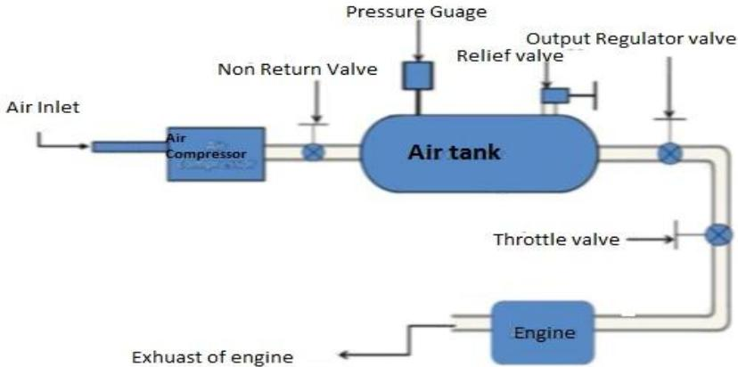
Figure 5: Line Diagram of Compressed Air Car
