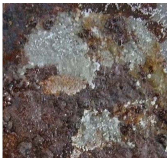
Figure 9: Complete failure of paint film after 40Hrs of exposure
