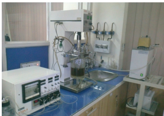
Figure 1 Fermentation of the isolate AI-6 in fermenter of 1.5 Liters.
